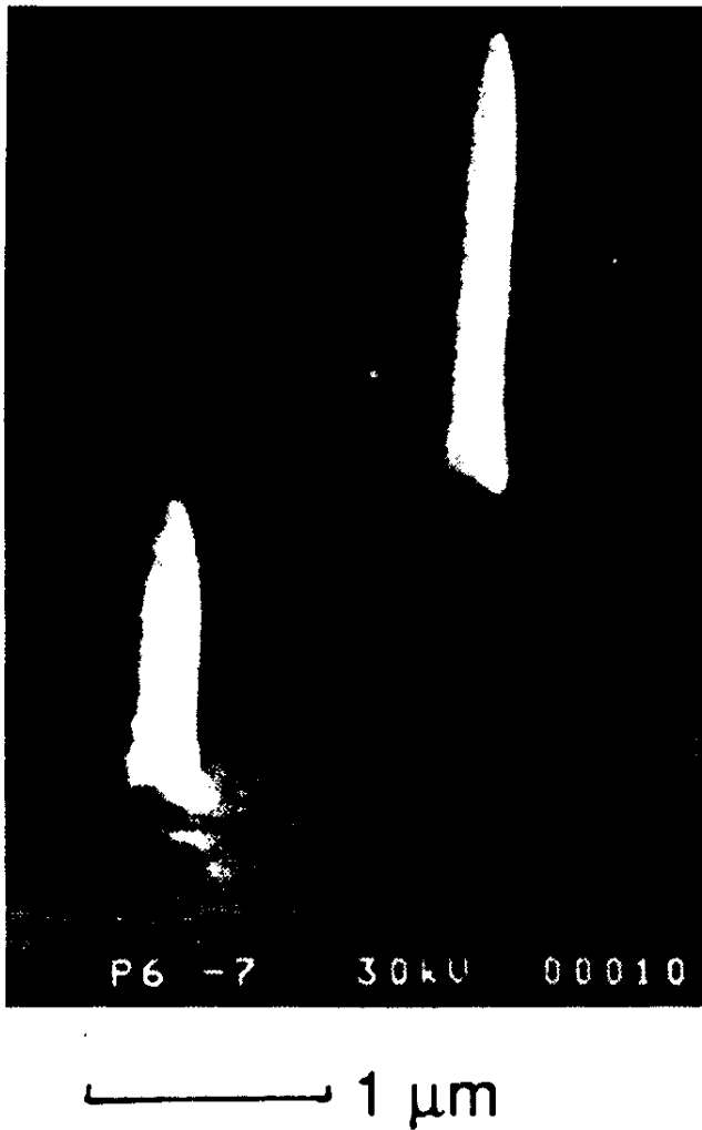
FIGURE 7.16 Electron-beam machining set-up and example of an electron-beam-formed W/C microstructure. (From Brunger, W.H. and Kohlmann, K.T., E-Beam-Induced Fabrication of Microstructures, presented at Micro Electro Mechanical Systems, Travemunde, Germany, 1992. With permission.)
