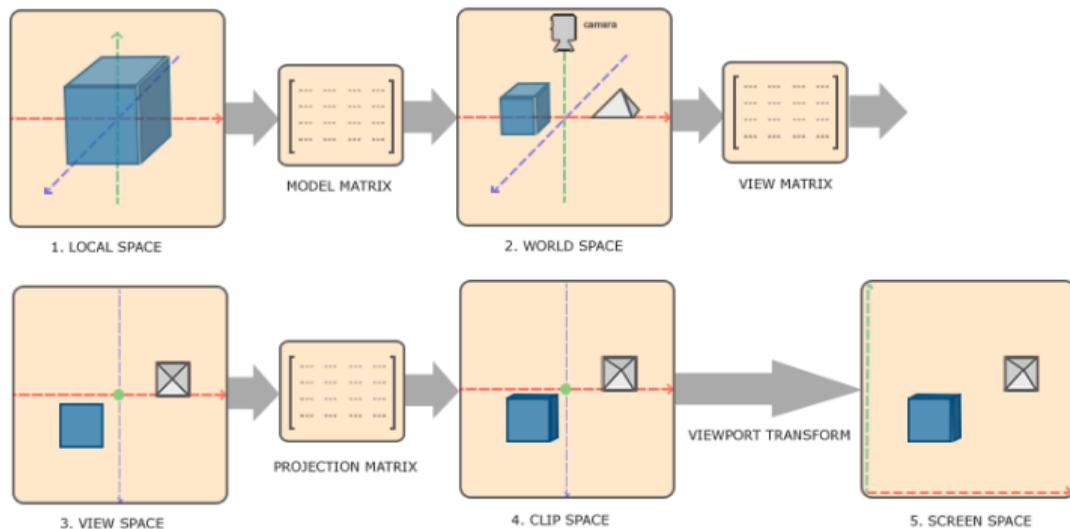
$$P' = \text{Projection} \times \text{View} \times \text{Model} \times P$$
