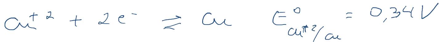
$$E_{\text{Cu}^{+2}/\text{Cu}} = E^{\circ}_{\text{Cu}^{+2}/\text{Cu}} - \frac{RT}{nF} \ln \frac{a_{\text{Cu}}}{a_{\text{Cu}^{+2}}}$$
