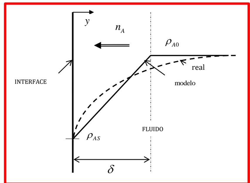
$$D_{AB} \frac{d^2 \rho_A}{dy^2} = 0 \quad \Rightarrow \quad \begin{cases} y = 0, & \rho_A = \rho_{AS} \\ y = \delta, & \rho_A = \rho_{A0} \end{cases} \quad \Rightarrow \quad \rho_A = \left( \frac{\rho_{A0} - \rho_{AS}}{\delta} \right) y + \rho_{AS}$$
