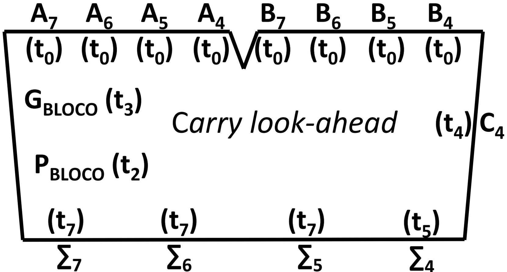
*Carry look-ahead* – Módulos 4 bits [3] –  $P_{\text{BLOCO}}$  e  $G_{\text{BLOCO}}$  –  $C_4$  Externo- obj
