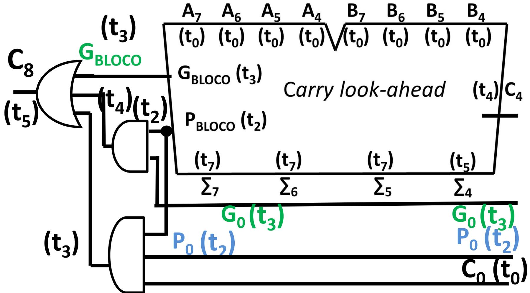
Carry look-ahead – Módulos 4 bits [1] e [2] –  $P_{\text{BLOCO}}$  e  $G_{\text{BLOCO}}$  –  $C_4$  Externo PNG
