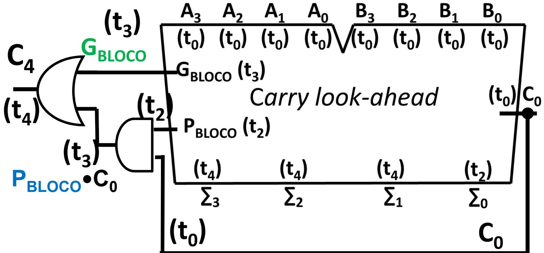
Carry look-ahead – Módulos 4 bits [2] –  $P_{\text{BLOCO}}$  e  $G_{\text{BLOCO}}$  –  $C_4$  Externo- obj PNG
