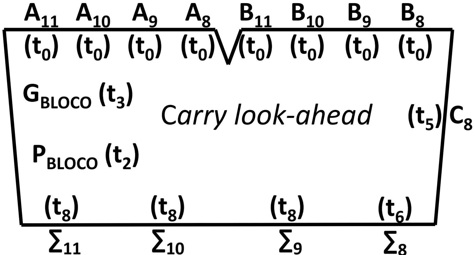
Carry look-ahead – Módulos 4 bits [1] –  $P_{\text{BLOCO}}$  e  $G_{\text{BLOCO}}$  –  $C_4$  Externo obj+PNG
