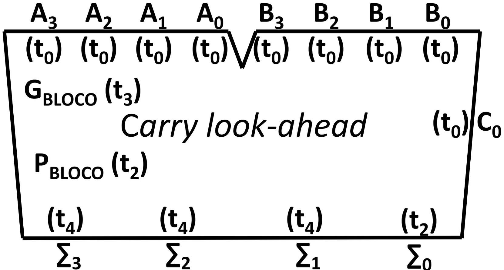
*Carry look-ahead* – Módulos 4 bits [2] –  $P_{\text{BLOCO}}$  e  $G_{\text{BLOCO}}$  –  $C_4$  Externo- obj
