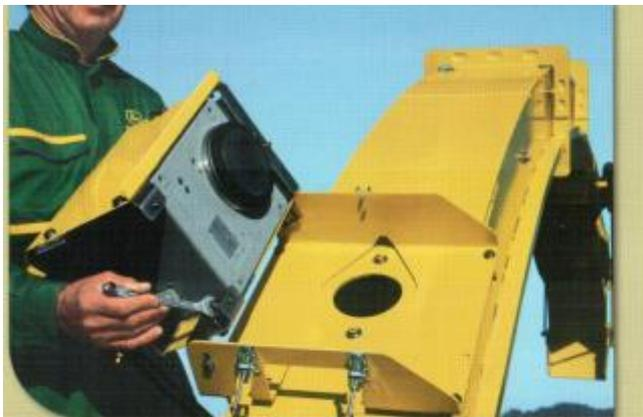
In the field, HarvestLab doesn't require calibration and can measure crop quality at material speeds of up to 40 m/sec. Thousands of measurements – on average one analysis per 50 kg of fresh silage – make readings more representative and accurate than with traditional methods.
