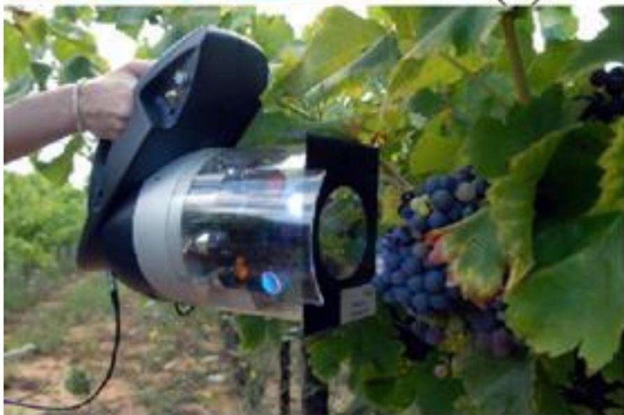
4 fontes de luz (LED): 373 nm (UV), 470 nm (B), 516 nm (G) e 635 nm (R)
