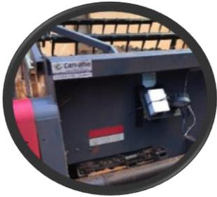
Cameras installed behind harvester platform
