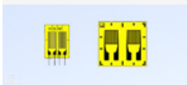
Strain gauge with 2 parallel measurement grids
