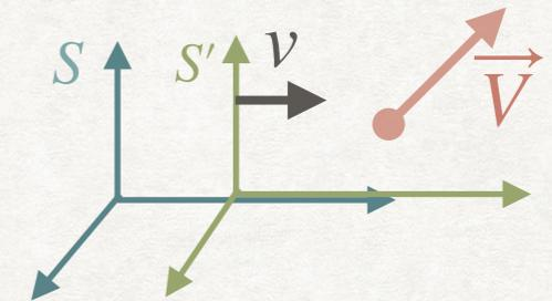
$$\begin{pmatrix} c dt' \\ dx' \\ dy' \\ dz' \end{pmatrix} = \begin{pmatrix} \cosh \theta & -\sinh \theta & 0 & 0 \\ -\sinh \theta & \cosh \theta & 0 & 0 \\ 0 & 0 & 1 & 0 \\ 0 & 0 & 0 & 1 \end{pmatrix} \begin{pmatrix} c dt \\ dx \\ dy \\ dz \end{pmatrix}$$
