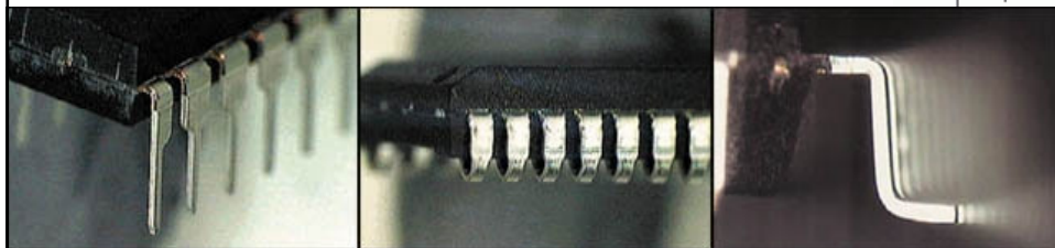
Figure 1. a) Straight lead, b) J-lead, and c) gull-wing lead.
