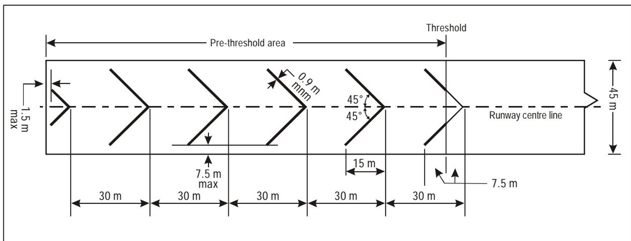
Figure 7-2. Pre-threshold marking
