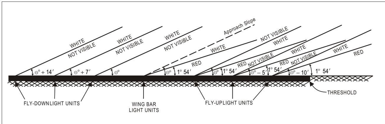
Figure 5-17. Light beams and elevation settings of T-VASIS and AT-VASIS
