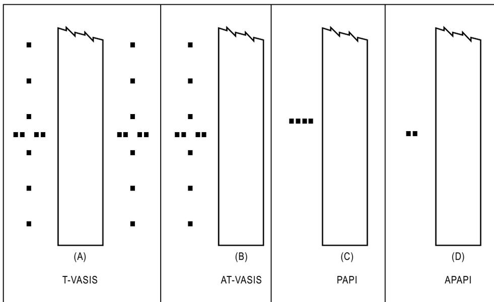
Figure 5-15. Visual approach slope indicator systems
