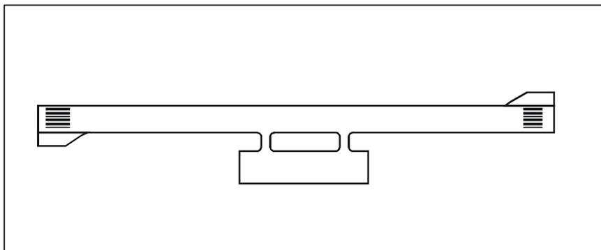
Figure 3-1. Typical turn pad layout
