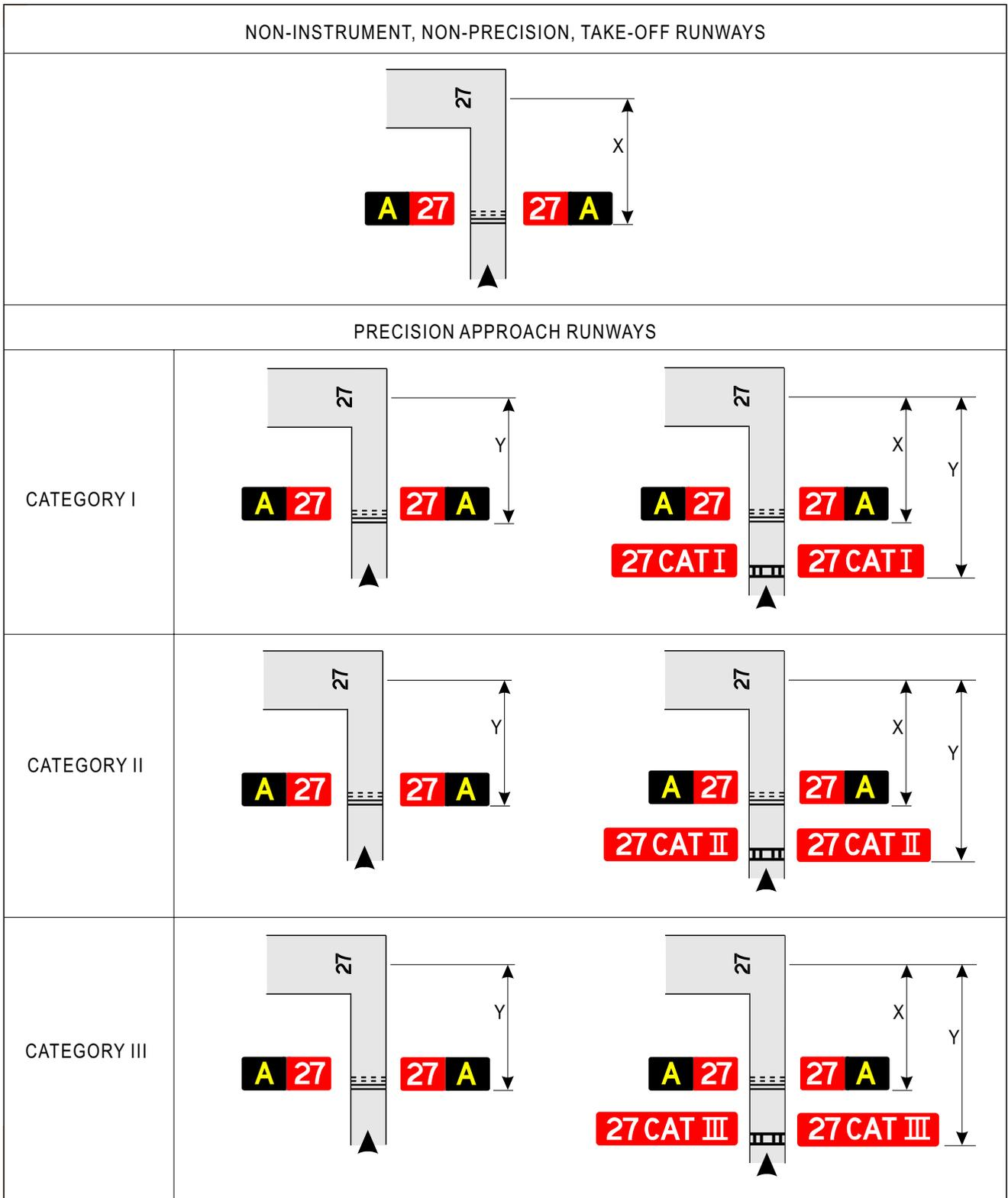
Note: Distance X is established in accordance with Table 3-2. Distance Y is established at the edge of the ILS/MLS critical/sensitive area.
