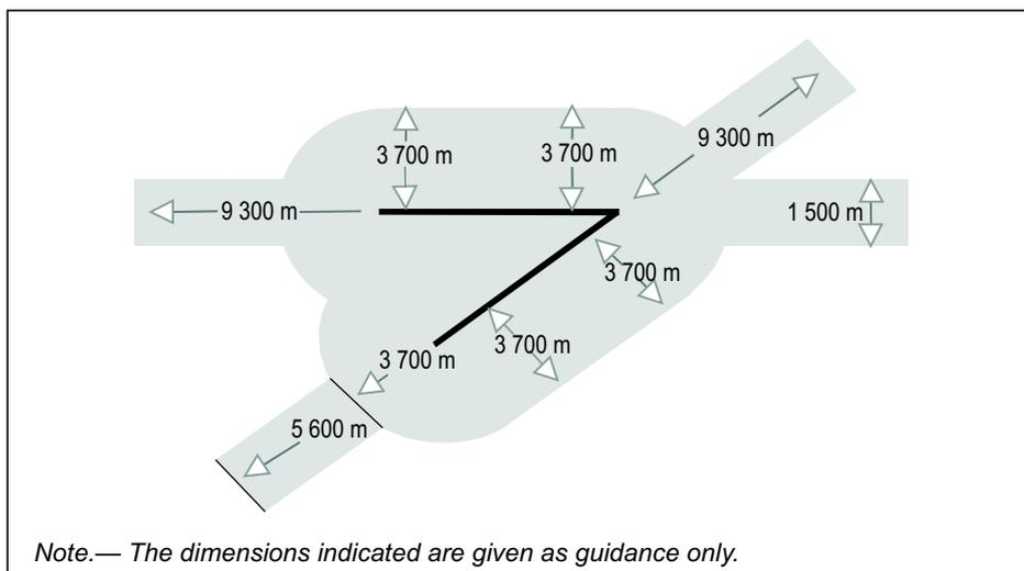
Figure 5-11. Multiple runway laser-beam free flight zone
