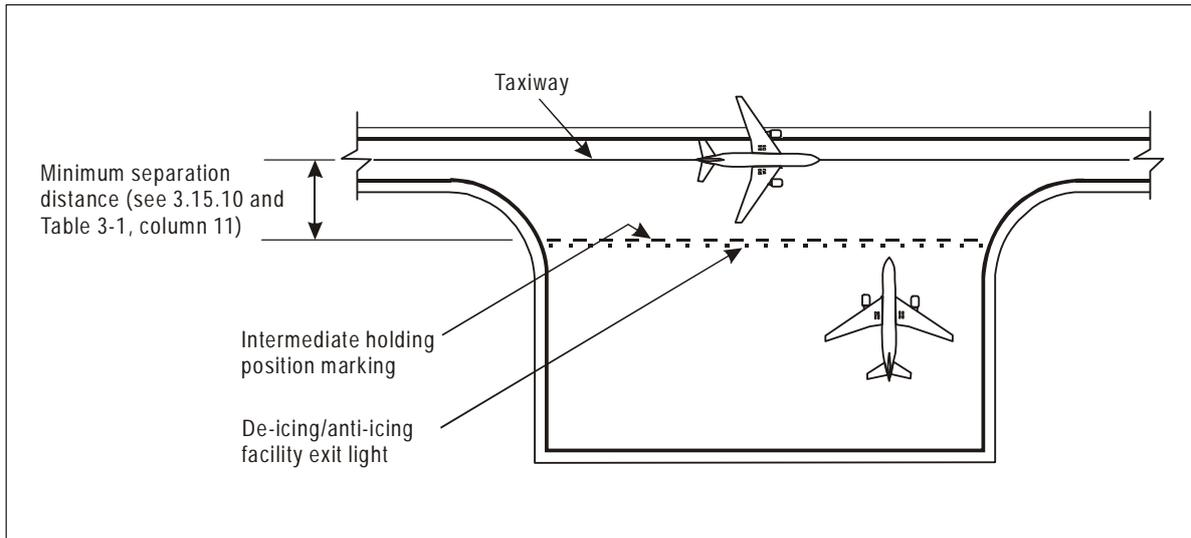
Figure 5-26. Typical remote de-icing/anti-icing facility
