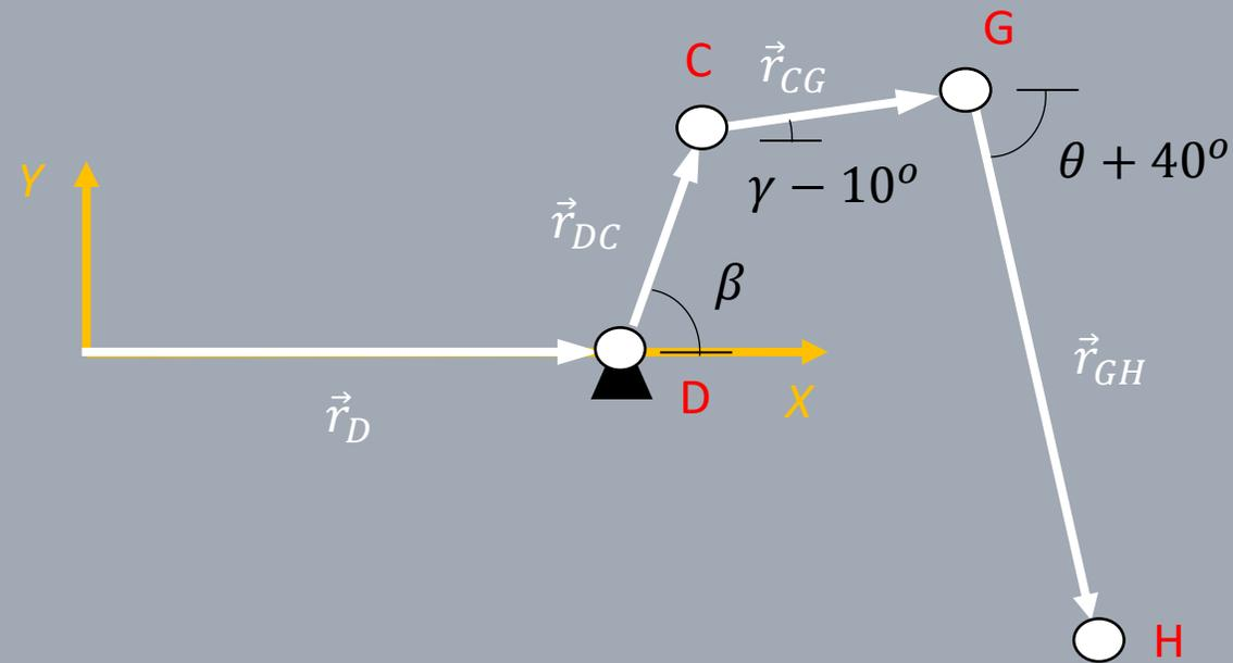
$$\begin{cases} x_H = x_D + L_{DC} \cos \beta + L_{CG} \cos(\gamma - 10^\circ) + L_{GH} \cos(\theta + 40^\circ) \\ y_H = L_{DC} \sin \beta - L_{CG} \sin(\gamma - 10^\circ) - L_{GH} \sin(\theta + 40^\circ) \end{cases}$$
