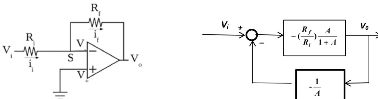
$$\frac{V_i - V_-}{R_i} = \frac{V_- - V_o}{R_f} \text{ (Lei de Ohm)}$$
