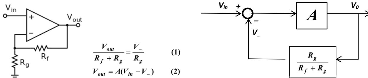
$$\frac{V_{out}}{R_f + R_g} = \frac{V_-}{R_g} \quad (1)$$
