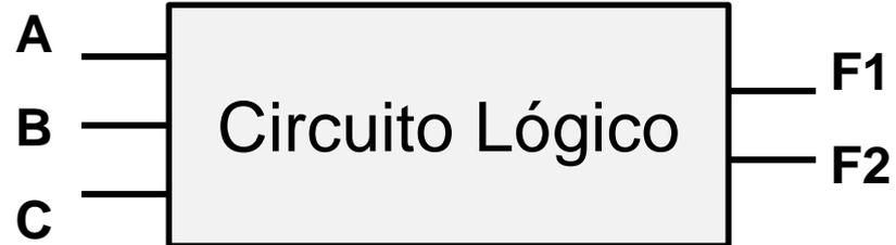
$$F1 = \overline{A}\overline{B}C + A\overline{B}\overline{C} + ABC$$
