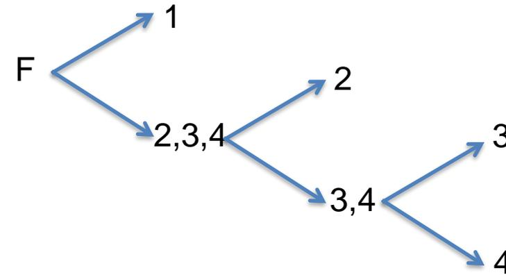
Separation of  $C$  components requires  $(C-1)$  distillation columns.
