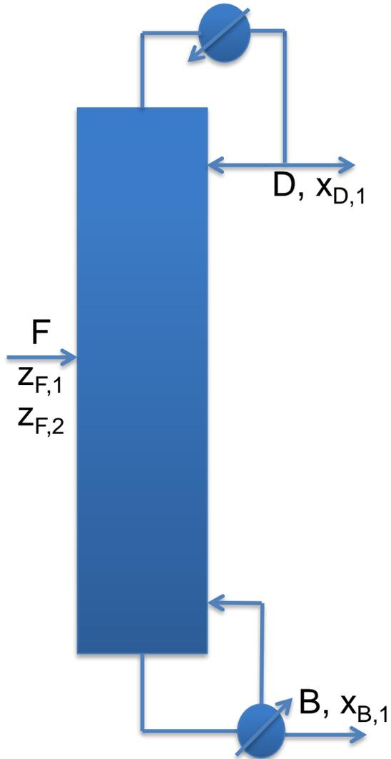
One distillation column can be optimized to separate one pair of volatile components.
