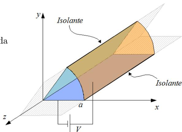
$$\nabla^2 \phi = 0 \Rightarrow \frac{1}{r} \frac{\partial}{\partial r} \left( r \frac{\partial \phi}{\partial r} \right) + \frac{1}{r^2} \frac{\partial^2 \phi}{\partial \theta^2} = 0; \quad \phi(r, \theta) \quad (1)$$
