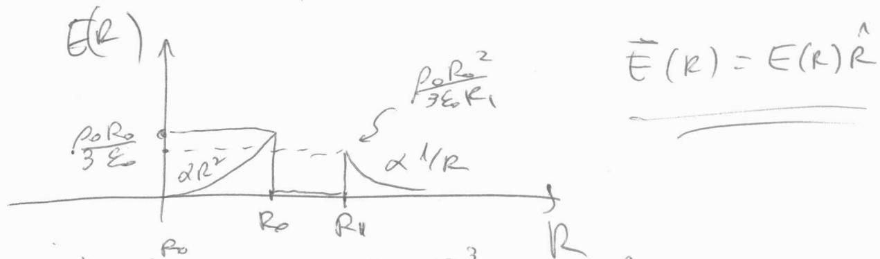
$$(b) V = \varphi(0) - \varphi(R_0) = \int_0^{R_0} E(R) dR = \frac{\rho_0 R_0^2}{3\epsilon_0} \frac{R_0^3}{3} = \frac{\rho_0 R_0^5}{9\epsilon_0} \quad -24$$
