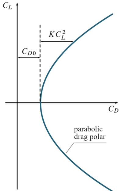
$$C_D = C_{D0} + KC_L^2 \quad K = \frac{1}{A Re \Pi}$$
