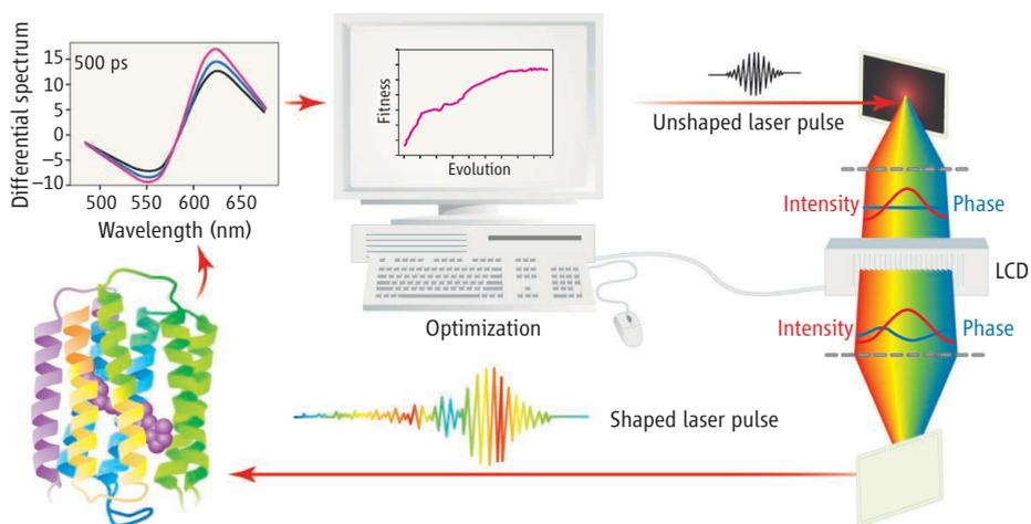
**In the loop.** A feedback loop is used to control isomerization of bacteriorhodopsin. An initial laser control field is created with a pulse shaper (on the right) and is then applied to the protein sample. The action of the control pulse, measured as the difference spectrum of the sample, is used by a learning algorithm to produce an improved field. Repeated excursions around the loop result in an optimum control.
