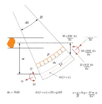
$\frac{\partial^2 M}{\partial x^2} + N \frac{\partial^2 w}{\partial x^2} + p(x, t) = m \frac{\partial^2 w}{\partial t^2},$
