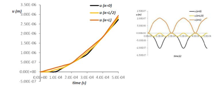
The next figure plots this solution for some specific parameters, a 10 mm diameter, 500 mm long aluminium bar under a force of 10 N. An inset is provided that shows only the vibrational motion, *ie* without the rigid body one.
