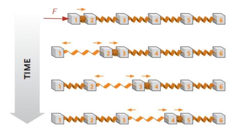
also evident from the previous figure that a longitudinal disturbance moving the particles in the same (opposite) direction it travels is a compressive (tensile) wave. Transverse movement of particles causes material shearing and the associate waves are called shear or torsional waves and are not considered here.
