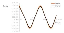
Motion of the extreme of a bar after a mass there connected is cut. In the examples above, loading was imposed to the bar via an initial condition. It was not necessary to have in the wave equation the force term, f(x,t). For a forced vibration however, f(x,t) comes into play and we need to solve the partial differential equation
