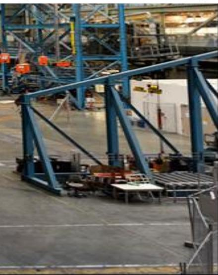
**PML's Mass and Force Group** calibrated the deadweights and load cells that Boeing used to help perform stress tests on the airframe of the 787 Dreamliner. Shown here is wing loading.
