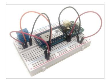
For the relay board, simply connect the VCC pin of the relay to Arduino VCC, GND to GND, and finally the SIG pin of the relay to Arduino pin 6. This is the final result:
