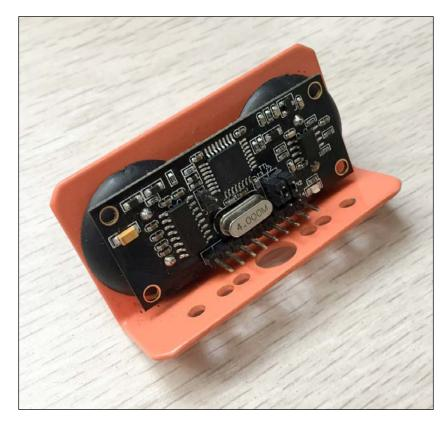
You can now mount the sensor on the robot's chassis, putting the sensor in front of the robot.
