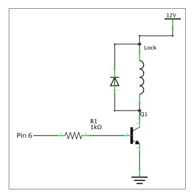
Make sure to follow the schematic to connect the door lock to the MKR1000 board, via the MOSFET transistor.
