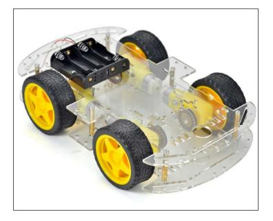
These are more stable than the two-wheeled platforms, but they are also more complex to control as you need to control four independent DC motors in the code of the Arduino board.
