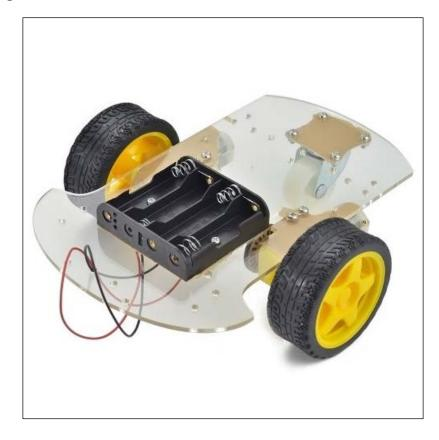
These platforms usually come with two motors already mounted on the robot, along with two wheels and a flywheel in front of the robot. They are easy to use, and you can usually mount an Arduino board on them.
