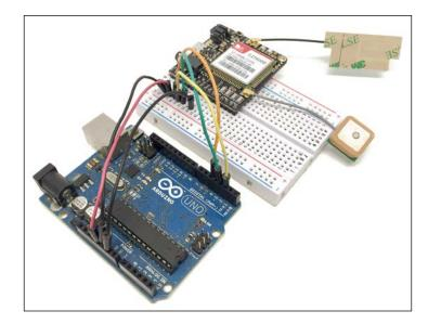
Just before using the project, also connect the battery to the  $\mathsf{GSM}/\mathsf{GPS}$  module via the JST connector.
