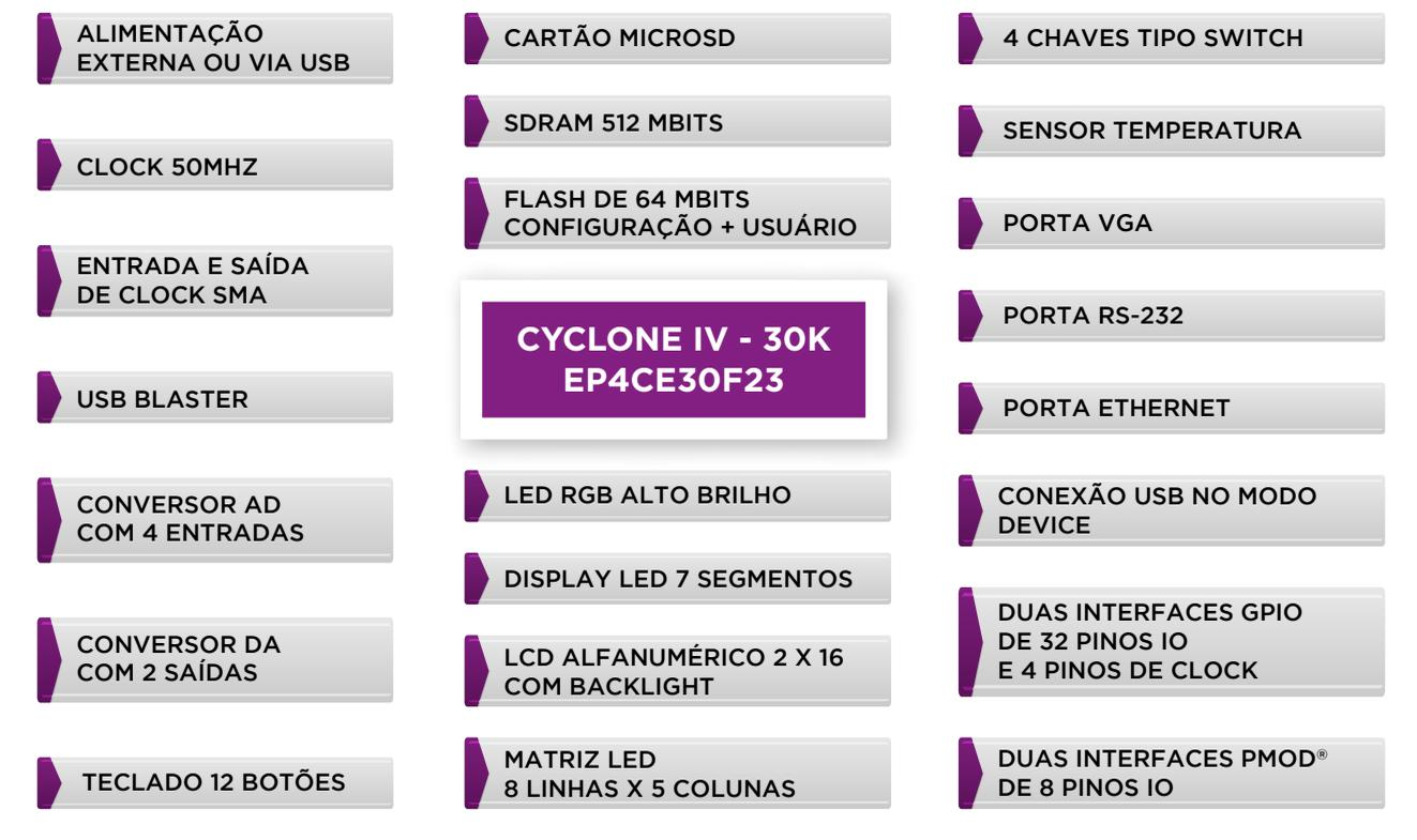
FIGURA 2 - DIAGRAMA DE BLOCOS DA PLACA MERCURIO® IV
