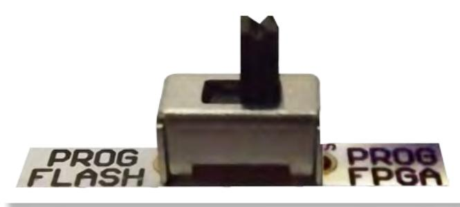
FIGURA 4 - CHAVE PROG NA POSIÇÃO FPGA
