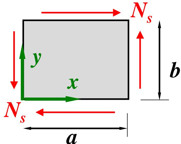
$$\frac{\partial^4 w}{\partial x^4} + \frac{\partial^4 w}{\partial x^2 \partial y^2} + \frac{\partial^4 w}{\partial y^4} + \frac{2N_s}{D} \frac{\partial^2 w}{\partial x \partial y} = 0$$
