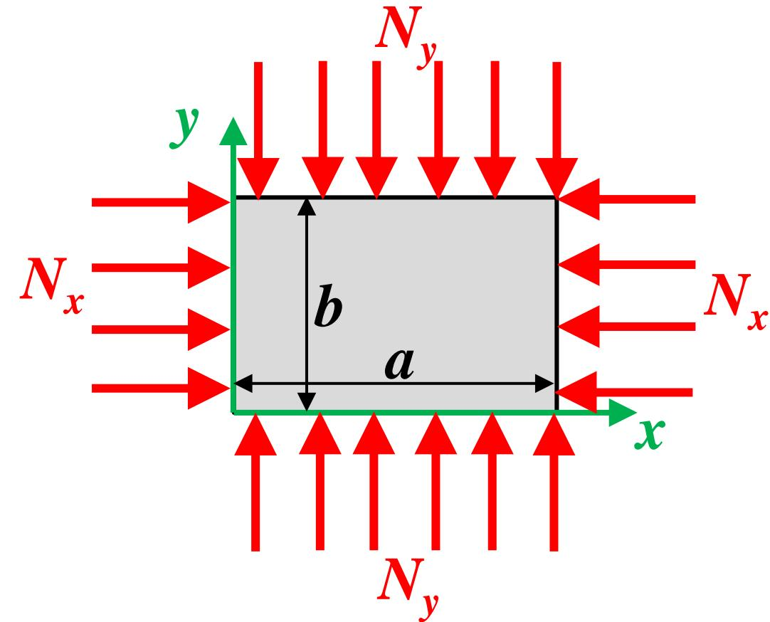
$$\frac{\partial^4 w}{\partial x^4} + 2 \frac{\partial^4 w}{\partial x^2 \partial y^2} + \frac{\partial^4 w}{\partial y^4} + \frac{N_x}{D} \frac{\partial^2 w}{\partial x^2} + \frac{N_y}{D} \frac{\partial^2 w}{\partial y^2} = 0$$
