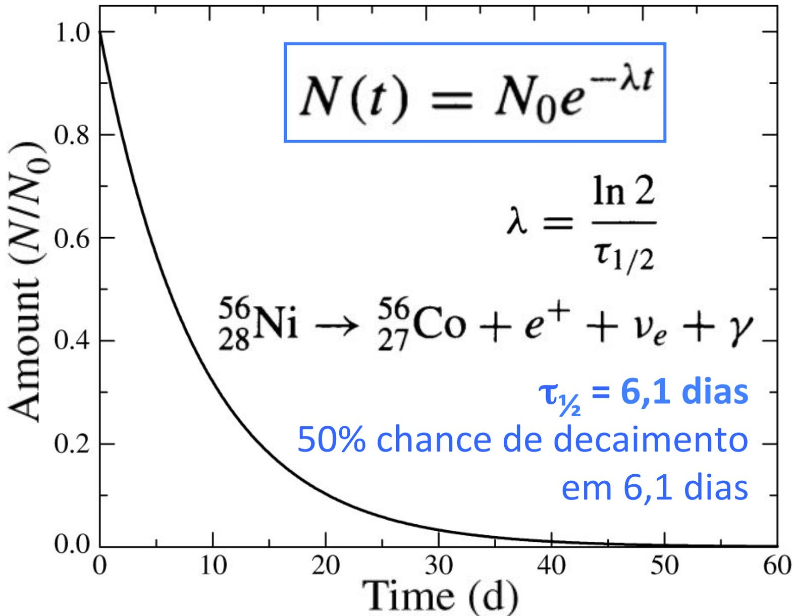
**FIGURE 15.11** The radioactive decay of  ${}^{56}_{28}\text{Ni}$ , with a half-life of  $\tau_{1/2} = 6.1$  days. There is a 50% chance that any given  ${}^{56}_{28}\text{Ni}$  atom will decay during a time interval of 6.1 days. If the original sample is entirely composed of  ${}^{56}_{28}\text{Ni}$ , after  $n$  successive half-lives the fraction of Ni atoms remaining is  $2^{-n}$ .
