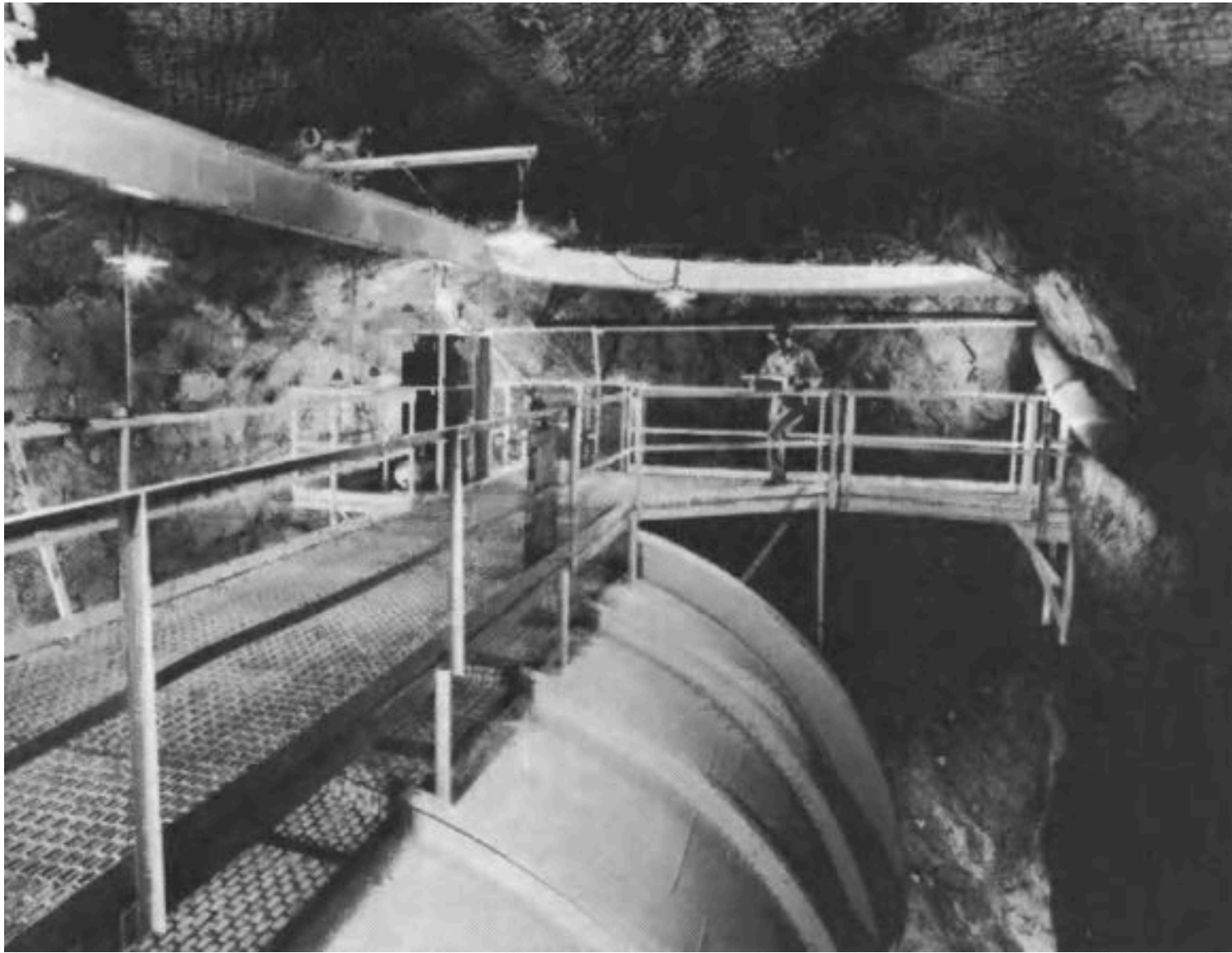
FIGURE 11.8 Raymond Davis's solar neutrino detector. The tank was located 1478 m (4850 ft) below ground in the Homestake Gold Mine in Lead, South Dakota, and was filled with 615,000 kg of C_2Cl_4 in a volume of 377,000 liters (100,000 gallons). (Courtesy of Brookhaven National Laboratory.)
