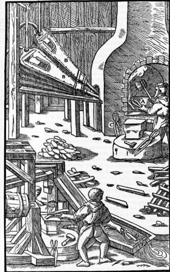
A—FORGE. B—BELLOWS. C—TONGS. D—HAMMER. E—COLD STREAM.
