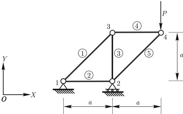
**Fig. 2.4.** A truss structure in the  $XY$  plane
