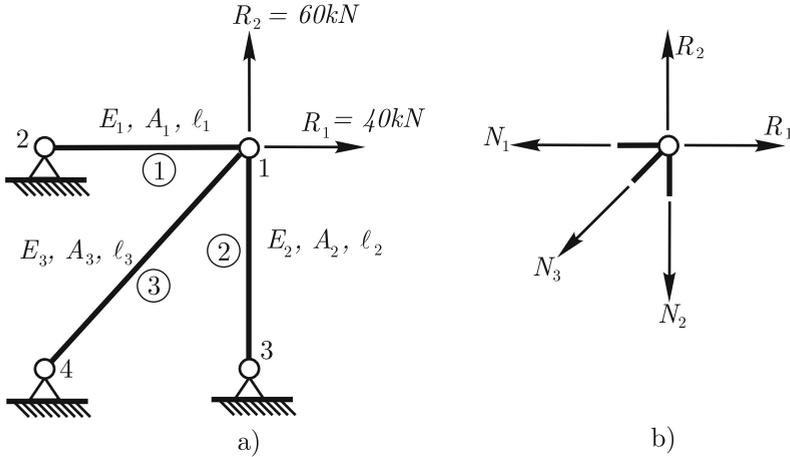
**Fig. 2.17.** a) Three-bar truss structure. The properties of bars 1 and 2 are as in Figure 2.16 and  $E_3 = 2.1 \times 10^{11} \text{ N/m}^2$ ,  $A_3 = 3A_1$ ; b) Equilibrium of node 1 for the three-bar truss
