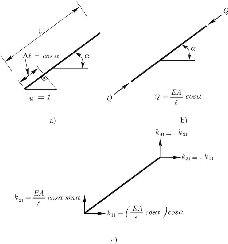
**Fig. 2.27.** Imposed horizontal unit displacement and corresponding forces. a) Imposed displacement and corresponding shortening of bar; b) Resulting force  $Q$  acting onto the bar; c) Nodal forces (stiffness coefficients) corresponding to (replacing) force  $Q$
