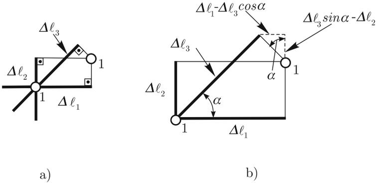
**Fig. 2.18.** Compatibility of displacements for node 1
