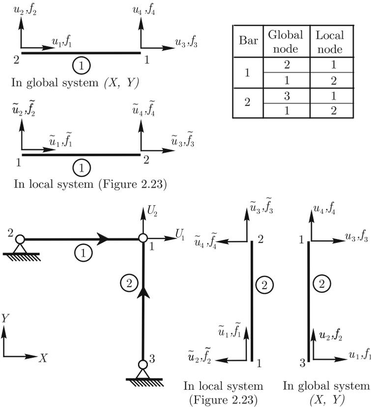
**Fig. 2.24.** Definitions for the two bar truss structure
