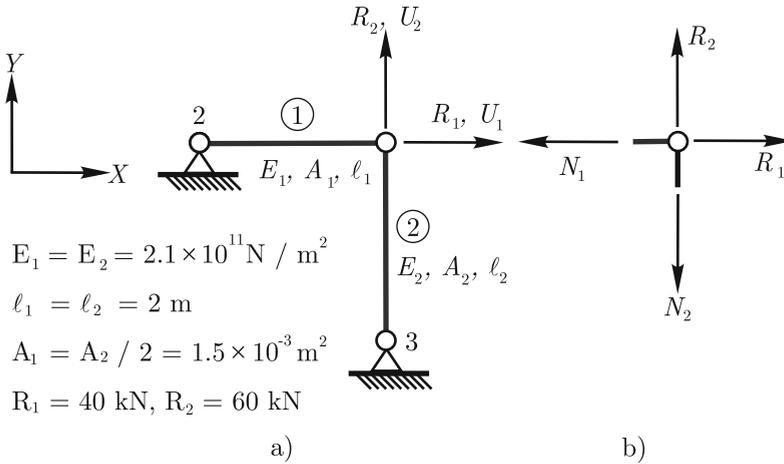
**Fig. 2.16.** a) Two-bar truss structure.  $R_1$  and  $R_2$  are concentrated applied loads and  $U_1$  and  $U_2$  are the node 1 displacements. Nodes and elements are numbered; b) Equilibrium of node 1 for the two bar truss
