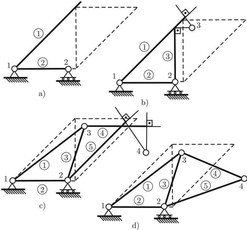
**Fig. 2.14.** Determination of the deformed configuration of a truss structure
