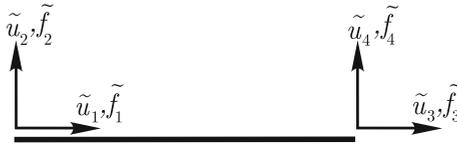
**Fig. 2.23.** Degrees of freedom of a truss bar
