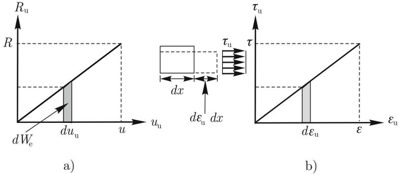
**Fig. 2.35.** a) Load displacement diagram for a truss bar; b) Stress-strain diagram for a generic point of a truss bar and side view of a differential volume element of the truss bar
