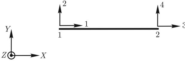
**Fig. 2.39.** One bar truss structure in X-Y plane
