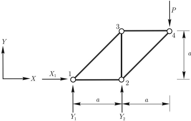
**Fig. 2.6.** Truss with reactions introduced explicitly
