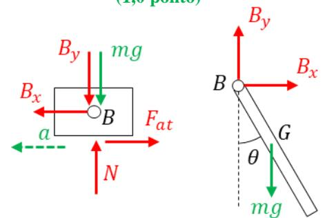
$$\vec{M}_B^{ext} = m(G - B) \wedge \vec{a}_B + (J_{Bz} \dot{\omega}) \vec{k}, \quad \vec{a}_B = -a \vec{i}, \quad J_{Bz} = \frac{mL^2}{3} \quad (1)$$
