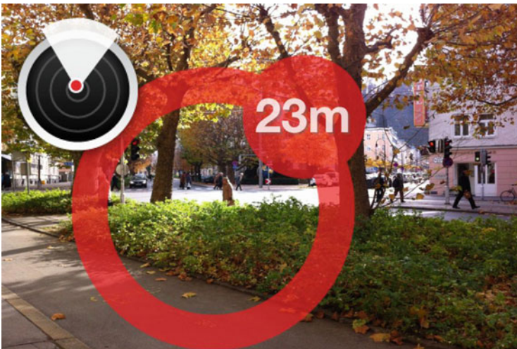
Fig. 11.2 A screenshot of the AR-based prototype, showing a ring. The distance to the next decision point is shown on the left of the ring to indicate a left turn at the current decision point
