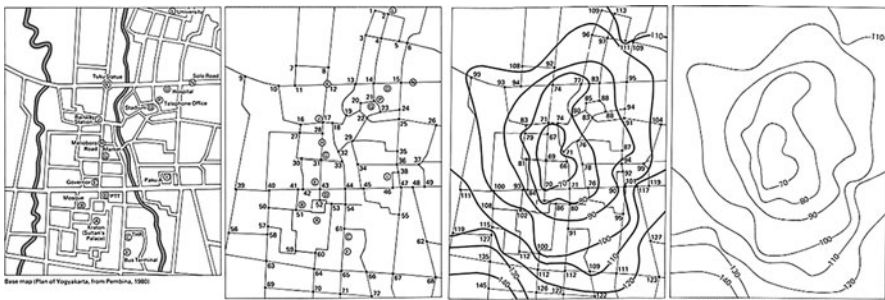
Fig. 2.5 Map exercise to assess the accessibility of urban services; the cumulative number of arcs it takes to get from each corner point to all public facilities is used as input for an accessibility isoline map (From Basic Cartography Exercise Manual (1991))
