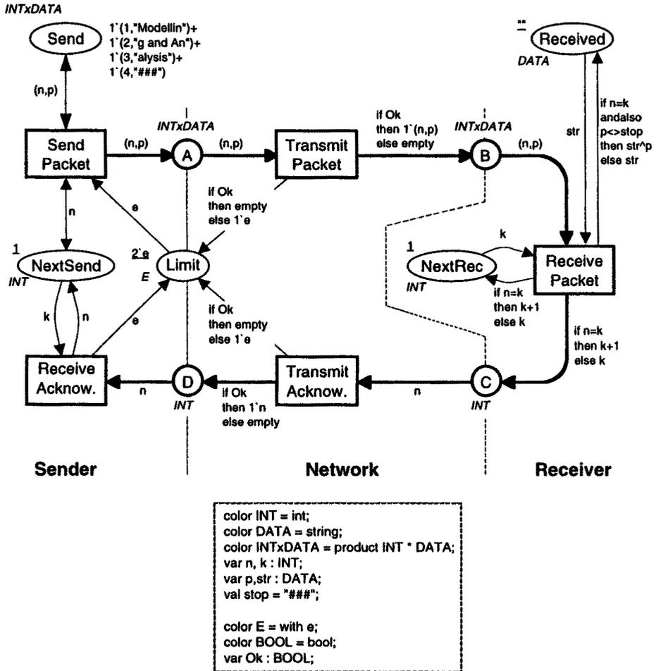
Fig. 16. Modified CP-net suitable for state space analysis
