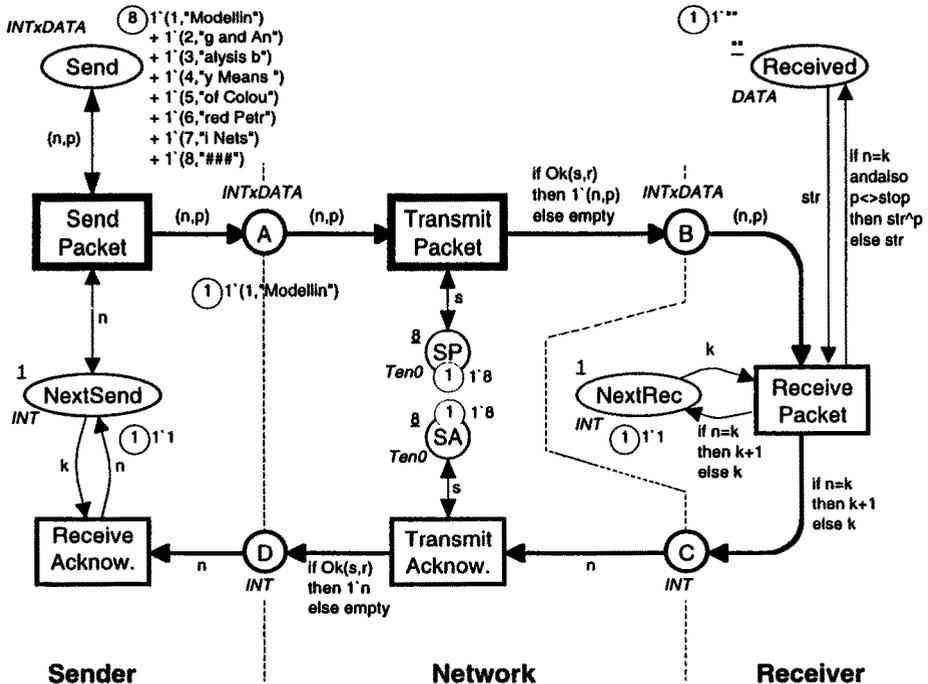
Fig. 3. Marking after occurrence of *Send Packet*
