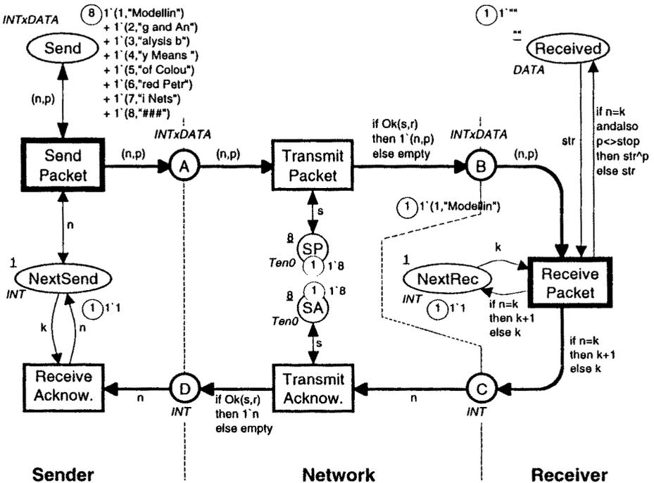
Fig. 4. Marking after occurrence of *Send Packet* and *Transmit Packet*
