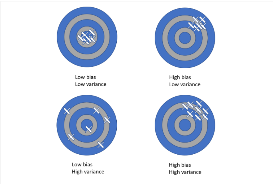
Figure 3-2. When taking samples of data, you need to be wary of four different levels of bias and variance that you could have
