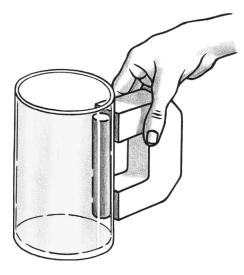
Fig. 4. A magnet presses a piece of iron against a glass. The attractive force between the magnet and the iron produces horizontal normal forces, which trigger vertical friction forces counteracting the weight of the iron pieces.
