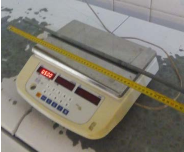
Figure 7.8. Weighting 60cm long 5/8 inch wire rod.
