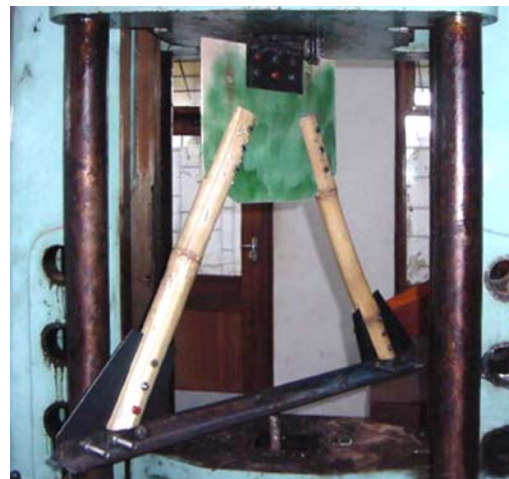
Figure 3.38. High ductility joint. Retrieved from Bamboo trusses with low cost and high ductility joints (p. 230) by M. Sassu, M. Andreini, A. De Falco & L. Giresini. Copyright Open Journal of Civil Engineering.
