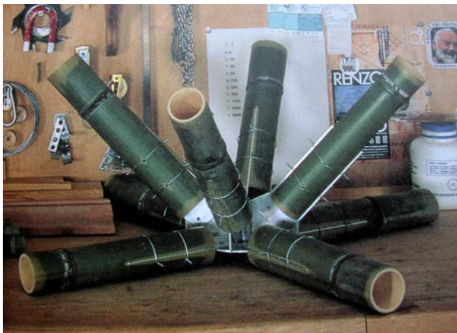
Figure 3.37. Bamboo joint designed by Renzo Piano. Retrieved from Traditional and innovative joints in bamboo construction (p.57) by A. Widyowijatnoko. 2012. PhD Dissertation at RWTH Aachen University.
