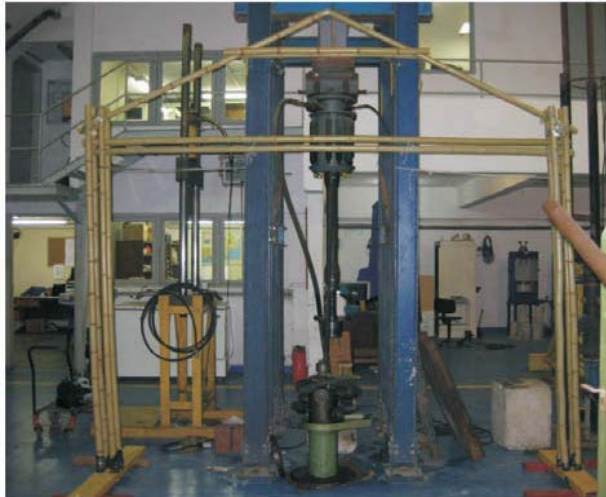
Figure 3.10. Mungpoo frame test. Retrieved from Performance based design of bamboo structure: Mungpoo frame test (p.7) by B. Sharma, K. Ghavami and K. Harries. 2011. International Wood Products Journal.
