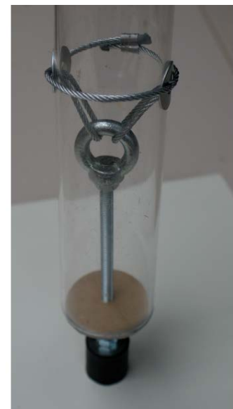
Figure 3.33. Design of a bamboo joint with eye-nut rod. Retrieved from Traditional and innovative joints in bamboo construction (p.92) by Widyowijatnoko. 2012. PhD Dissertation at RWTH Aachen University.
