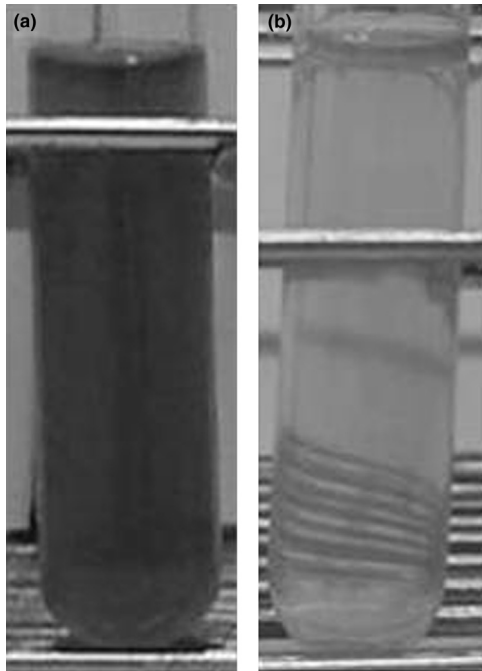
Figure 6 Visual judgment of the samples (a) positive and (b) negative for guaiacol. Considering a gray scale of colors, light gray refers to negative results and dark gray refers to positive results.
