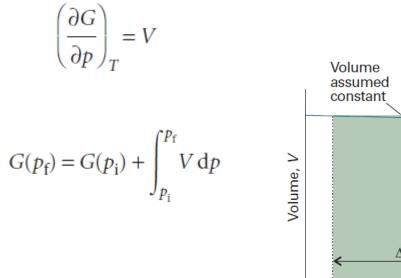
Volume assumed constant  $\Delta p$  $p_i$  $p_r$ Pressure, p Condensed phase (liquids and Solids) changes  $V_{\rm m}$  is almost constante
