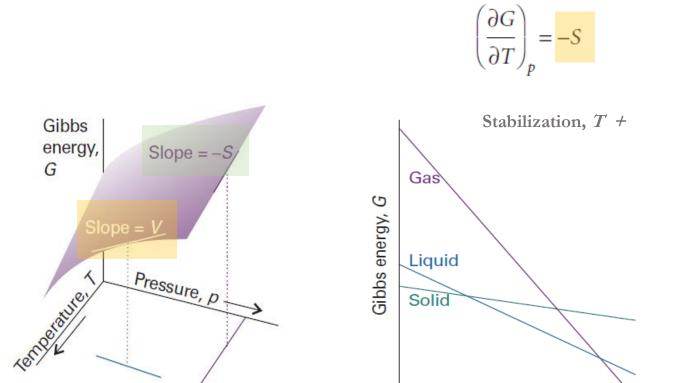
$\left(\frac{\partial G}{\partial p}\right)_T = V$ destabilization,  $p \neq 0$
