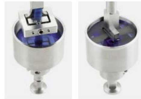
Sample holder for tensile tests (left) and bending tests (right) in an immersion bath
