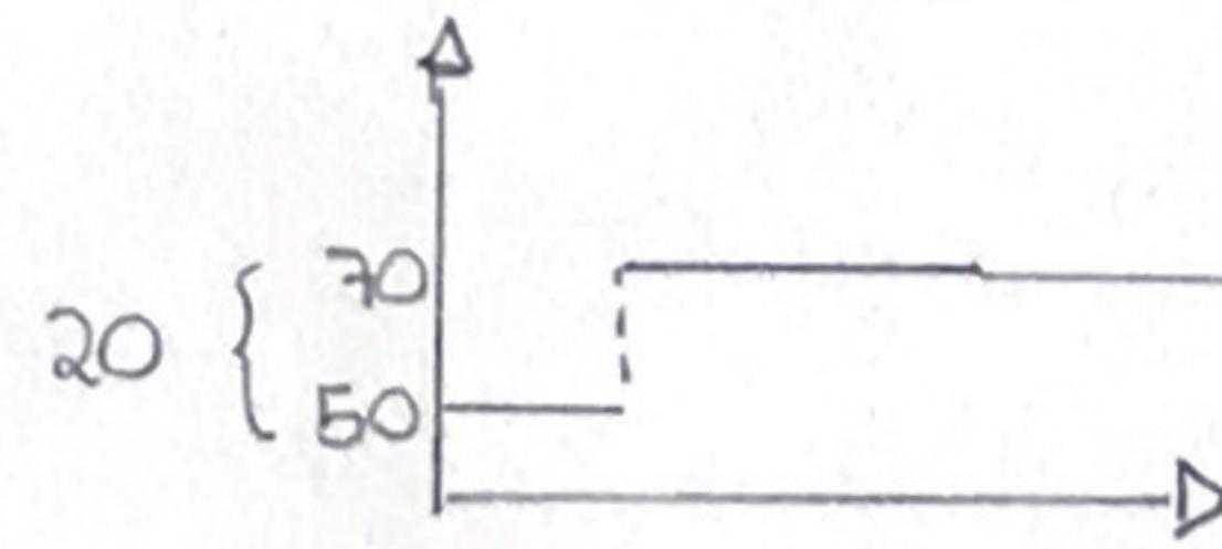
$$20 \frac{\text{gal}}{\text{min}} \cdot \frac{1,3368 \cdot 10^{-1} \text{ ft}^3}{1 \text{ gal}} = 2,68 \frac{\text{ft}^3}{\text{min}} \quad \therefore \quad \bar{h}(s) = \frac{0,90}{11,32s+1} \cdot \frac{2,68}{s}$$
