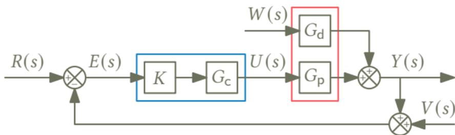
$$Y(s) = \underbrace{\frac{KG_c(s)G_p(s)}{1 + KG_c(s)G_p(s)}}_{T(s)} (R(s) - V(s)) + \underbrace{\frac{1}{1 + KG_c(s)G_p(s)}}_{S(s)} G_d(s)W(s)$$
