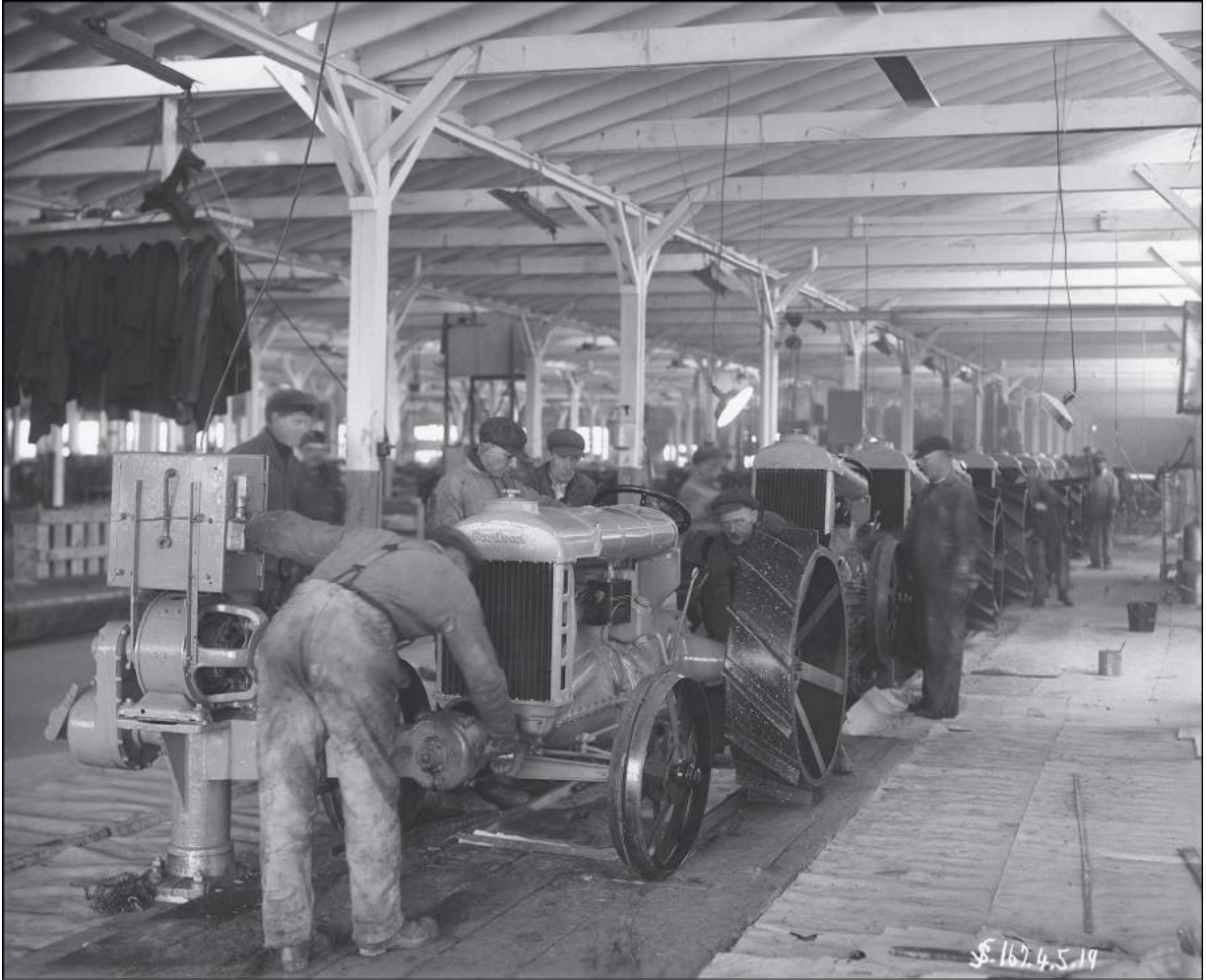
16. According to Henry Ford, "The motor enabled machinery to be arranged according to the sequence of the work, and that alone has probably doubled the efficiency of industry..." This is his Rouge Plant in 1919, with electricity throughout.
