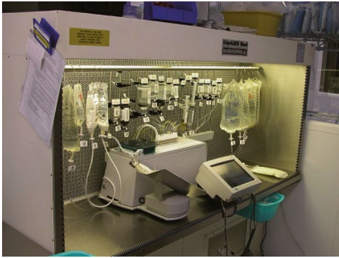
Figure 21.6 An automated compounder used for preparing parenteral nutrition solutions at the University of California, San Diego Medical Center.
