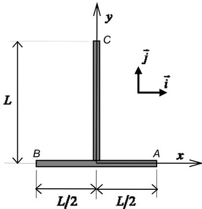
$$\vec{V}_A = \frac{\omega L}{2} \vec{j}, \quad \vec{V}_B = -\frac{\omega L}{2} \vec{j} \quad \text{e} \quad \vec{V}_C = -\omega L \vec{i} + \omega L \vec{k}$$
