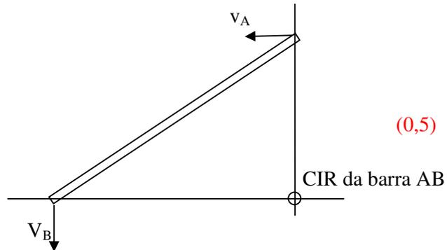
$$\vec{v}_B = \vec{\omega}_{AB} \wedge (B - CIR_{AB}) = \omega_{AB} \vec{k} \wedge (-L_1 \cos \theta \vec{i}) \Rightarrow \boxed{\vec{v}_B = -\omega_1 R_1 \cot \theta \vec{j}} \quad (0,5)$$
