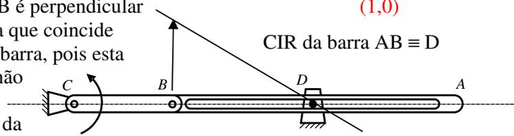
$$\vec{v}_B = \vec{\omega}_2 \wedge (B - D) \Rightarrow \omega_1 R \vec{j} = \omega_2 \vec{k} \wedge (-L \vec{i}) \Rightarrow \omega_2 = -\omega_1 \frac{R}{L} \Rightarrow \boxed{\vec{\omega}_2 = -\omega_1 \frac{R}{L} \vec{k}} \quad (0,5)$$
