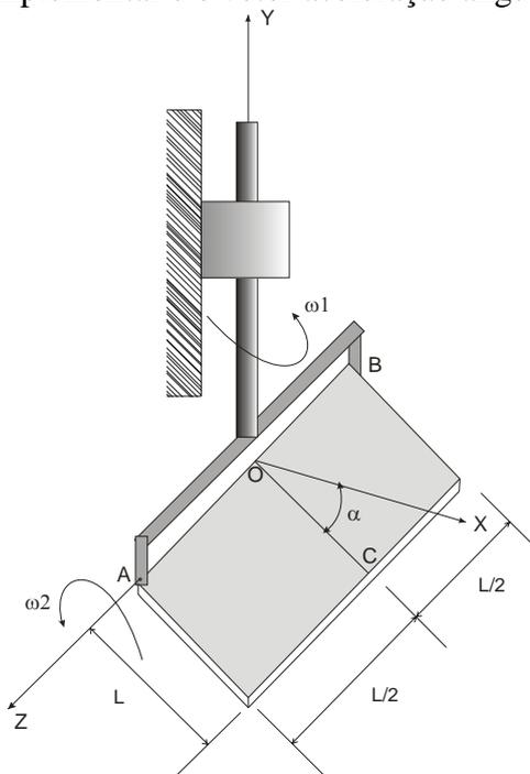
$$a) \vec{V}_{C,rel} = \omega_2 \vec{k} \wedge L \frac{\sqrt{2}}{2} (\vec{i} - \vec{j}) = \omega_2 L \frac{\sqrt{2}}{2} (\vec{i} + \vec{j})$$
