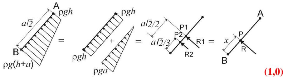
$$R_1 = \gamma ah\sqrt{2}L ; R_2 = \frac{1}{2}\gamma a^2\sqrt{2}L$$
