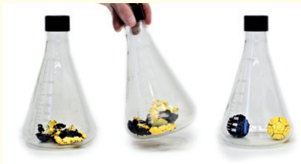
Figure 9. Demonstration of self-assembly and molecular chirality, or right-handed and left-handed patterns of attraction. Opposing attraction patterns in the self-assembly units allowed for the parts to sort themselves when combined and shaken randomly. The yellow units and black units eventually self-assemble into two distinct structures, demonstrating error-correction throughout the assembly process. The molecular structures in this exhibit were based on the Polio Virus capsid.
