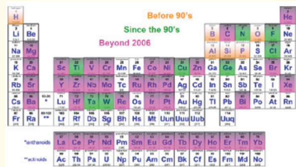
Figure 10. Elements employed in Si technology. Up to 1990, the fabrication of Si-based electronics involved merely 6 elements, namely Si as the fundamental semiconductor material, B and P for doping, O for making insulating layers, H for passivation, and Al for the interconnects. In the next decade the basic six elements were complemented by Ti, Ta, W, Cu, Ge, N, F, and Cl. Today, approximately 50 elements, in particular also rare earth elements, are used in the manufacturing process.
