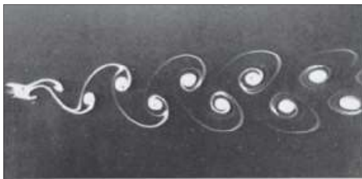
Fig. 3.2 Streaklines in the unsteady flow around a cylinder. (Photography by Sadatoshi Taneda. From Album of Fluid Motion, 1982, The Parabolic Press, Stanford, California.)
