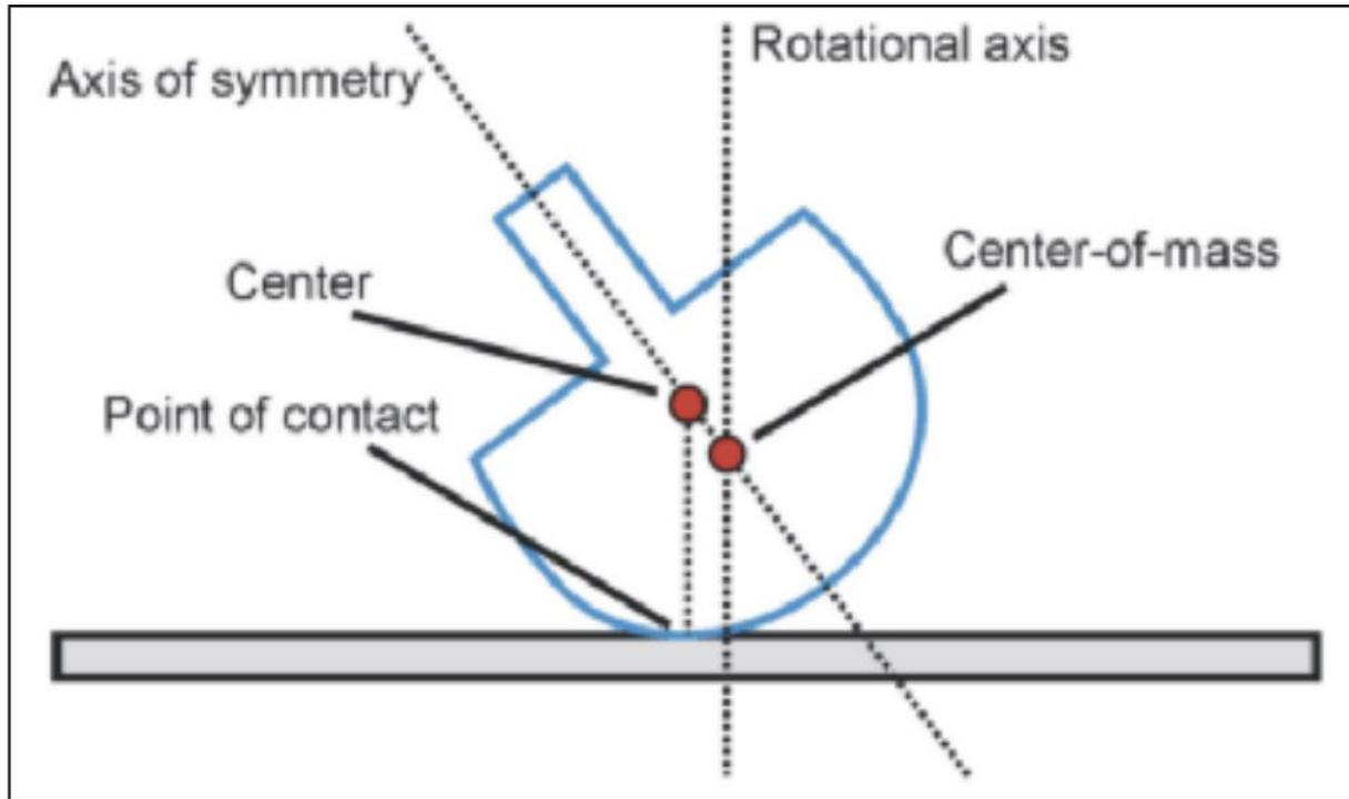
*Since the geometrical center of the sphere does not coincide with the center-of-mass, the point of contact with the surface will not coincide with the rotational axis.*
