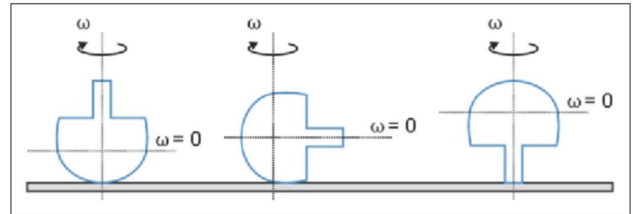
Rotational axes of a Tippie Top. When the top is almost (not completely) horizontal, the rotation around the stem will stop and start to rotate the other way.
