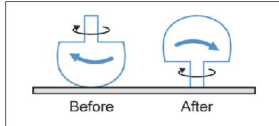
The Tippie Top is a spinning top, which will automatically lift its center of mass while it starts to turn in the opposite direction.
