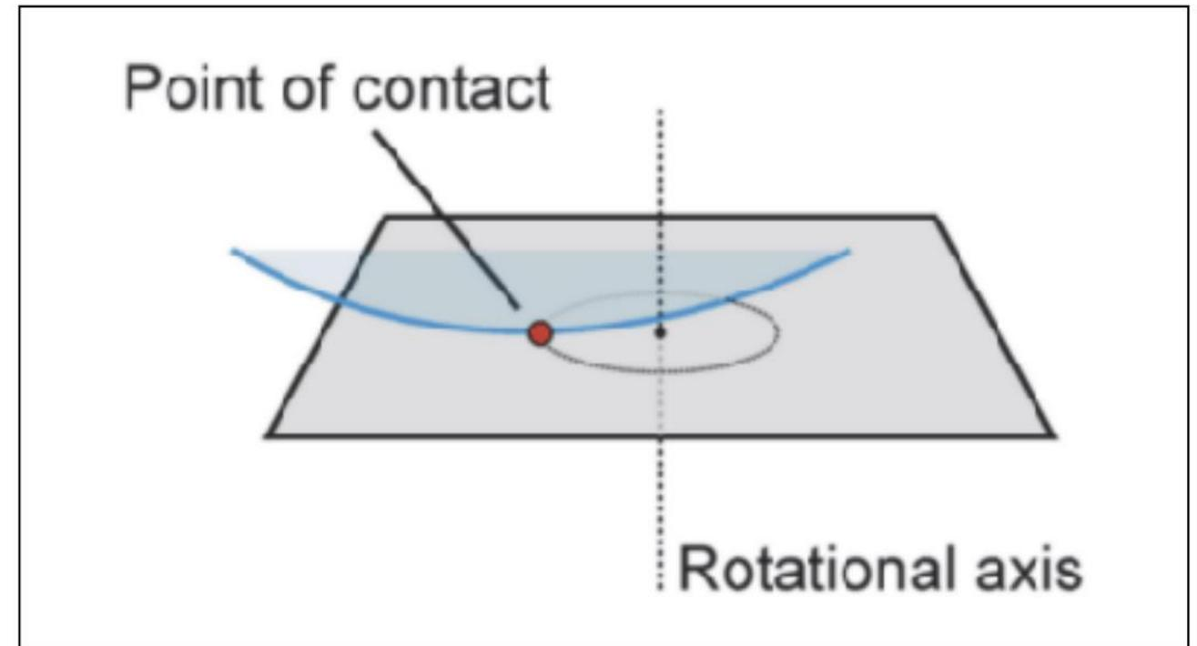
*Since the point of contact does not coincide with the rotational axis, the Tippe Top will slide over the surface in a circle around the rotational axis. The sliding friction supplies the torque needed for the inversion of the top.*
