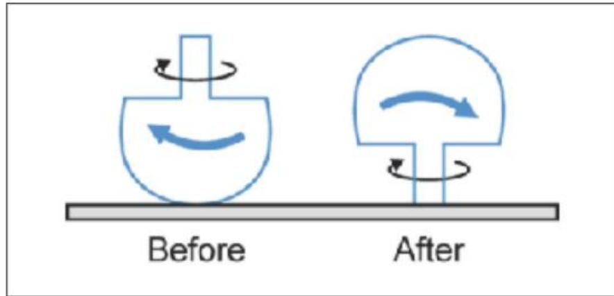
*The Tippe Top is a spinning top, which will automatically lift its center of mass while it starts to turn in the opposite direction.*
