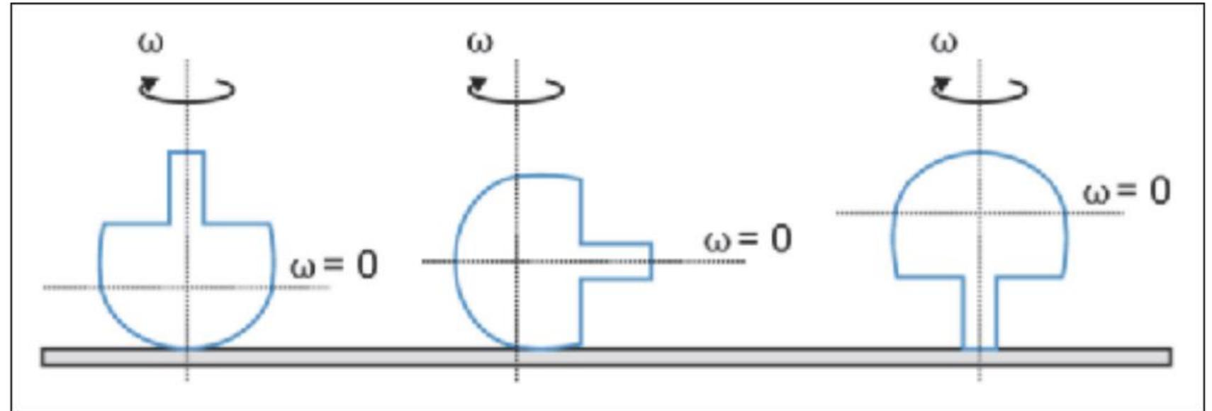
*Rotational axes of a Tippe Top. When the top is almost (not completely) horizontal, the rotation around the stem will stop and start to rotate the other way.*
