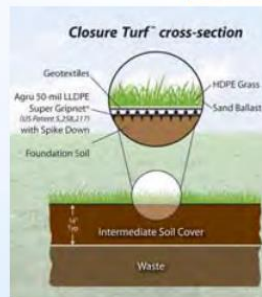
Sand is applied as a ballast eliminating the need for anchoring.
