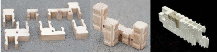
Fig. 8: SL block CNC milled from cross-laminated veneer plywood elements and a demonstrator element made from planar material of varying thicknesses.
